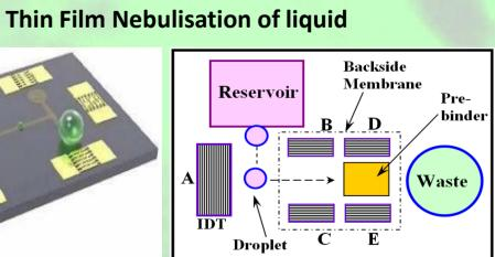
Acoustic wave based lab-on-chip
