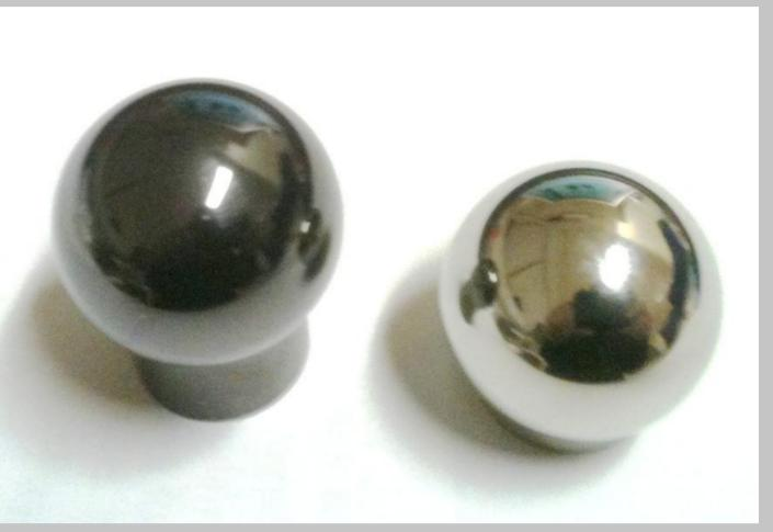
Hip joint test pieces: right image is uncoated Ti alloy, left is DLC coated
