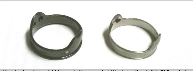
Heart valve rings: right image is the uncoated titanium alloy, left is DLC coated
