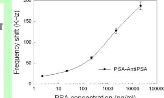
PSA concentration (ng/ml) Acoustic wave based biosensing
